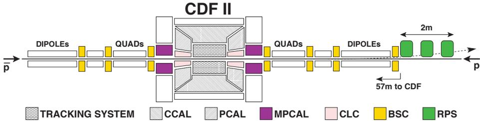
Fig. 3. Schematic drawing of the CDF II detector and beam layout (Ref. 11).
